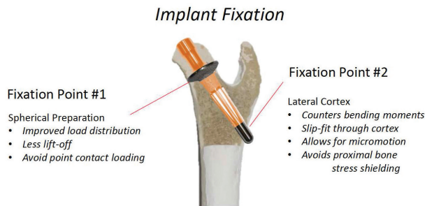
Figure 6 —Design concept showing placement of Centerline THA within the proximal femur. Figure courtesy of Biomedtrix.
